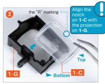
Turn the **Headlamp Lens (R)1-C** upside down, orient the notch downward, and set it onto the inner projection of part **1-G**.
