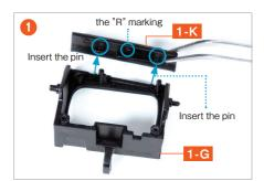
Insert the two pins of the **Headlamp Housing (R)1-G** into the circled holes of
