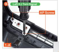
Align the screw holes and fit the left turn signal assembly from step into the square hole on the left side of the back of **Front Bumper 1-A**. Fasten it with AP screws at the two positions shown.
