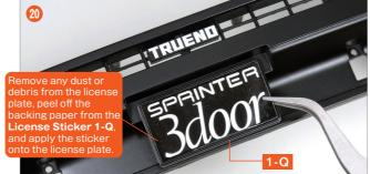
Remove any dust or debris from the license plate, peel off the backing paper from the **License Sticker 1-Q**, and apply the sticker onto the license plate.
