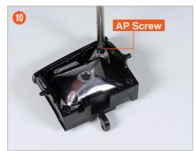
Align the screw holes and fasten with one **AP screw**.
