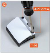
While holding the parts from step (1) to prevent them from coming apart, turn the assembly over, align the screw holes, and fasten with AP screws at the two positions as shown.
