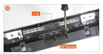
While holding the license plate to prevent it from coming loose, turn the front bumper over and fasten it with **AP screws** at the two positions as shown.
