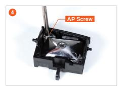
Align the screw holes and fasten with one **AP screw**.
