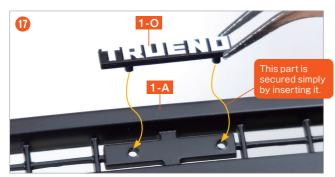
Insert the pins of the **TRUENO Emblem 1-O** into the center hole of the grille on **Front Bumper 1-A**, orienting it as shown.
