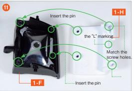
Place the Retractable Headlamp Cover (L)1-H over the assembly from step ①.
